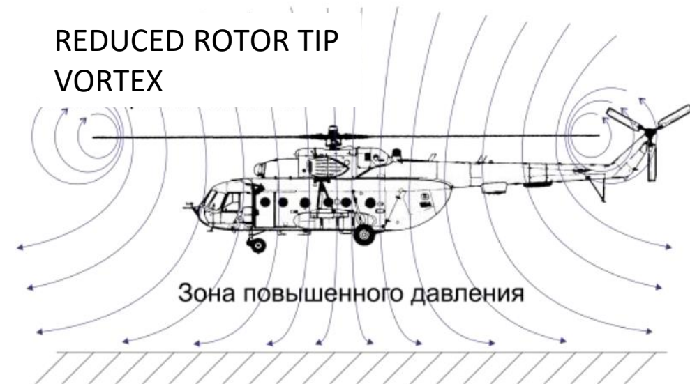
Fig. 9.17. Airflow when in ground effect
